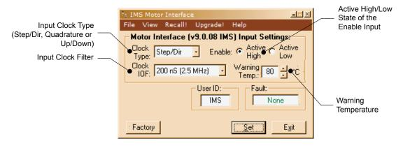
Figure 2.6.8: SPI Motor Interface I/O Settings Screen
